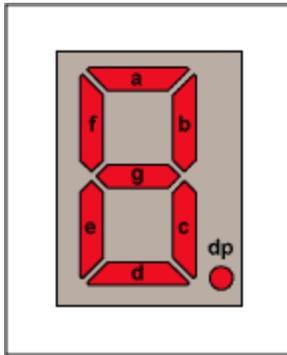
Figure 2. Segment labeling for 7-segment display.
