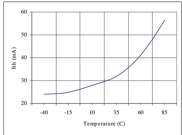
Figure 2. Laser threshold change over temperature
