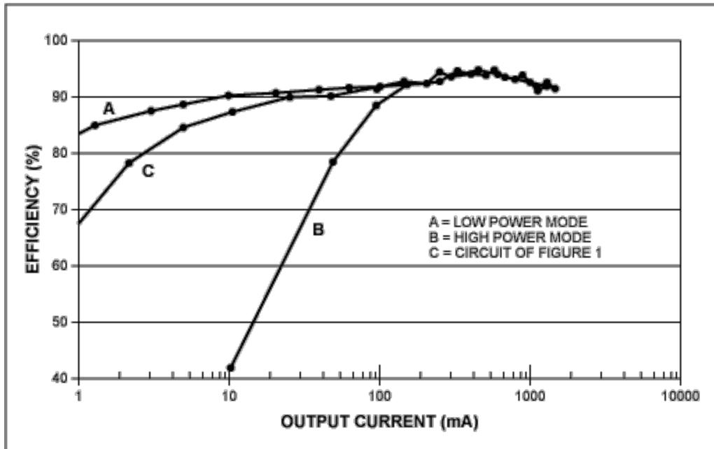
Figure 2. The Figure 1 circuit's conversion efficiency (C) remains high for a wide range of load current.
