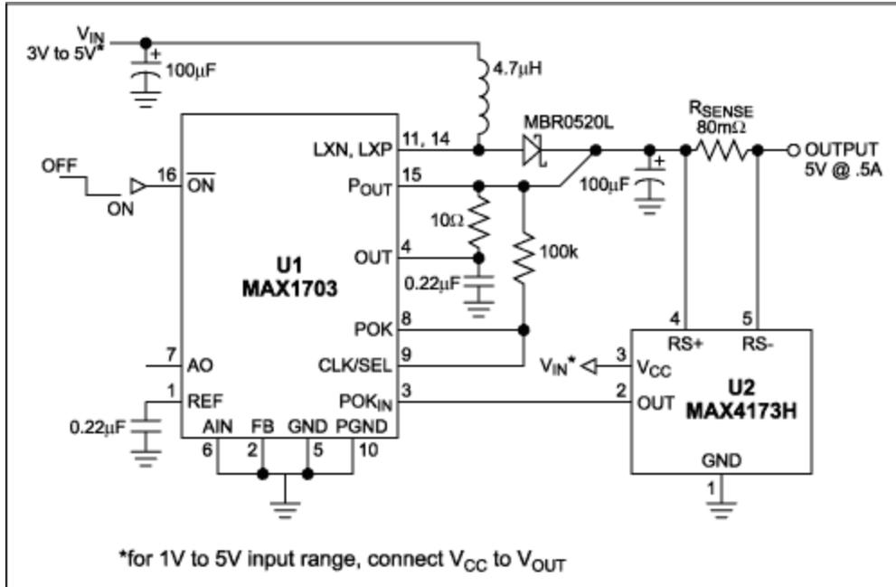
Figure 1. Using a high-side current monitor (U2) to generate a proportional feedback voltage, this synchronous boost converter (U1) shifts automatically between its high-power and low-power modes of operation.
